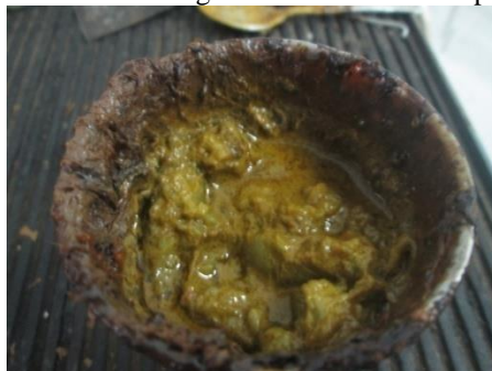
Figure 6. A mixture of bacterial cellulose fiber-shellac with alcohol solvent
