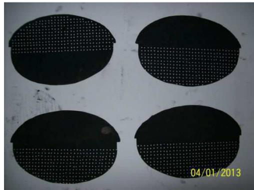
Gambar 2. Material Substrat Berlapis Mangan Model 3
