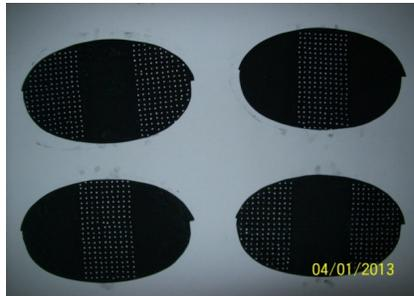
Gambar 2. Material Substrat Berlapis Mangan Model 2
