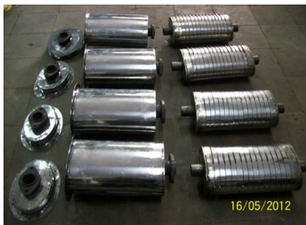
Gambar 3. *Chasing Catalytic Converter*
