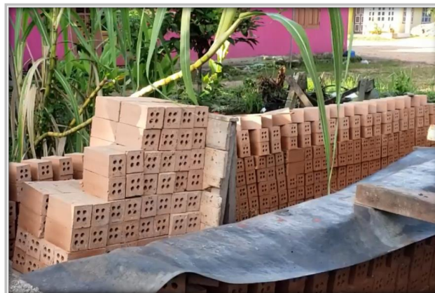
Figure 10. Difference between wet brick and dry brick
