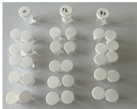
Figure 1. Specimen after being filled with saliva solution according to the concentration
