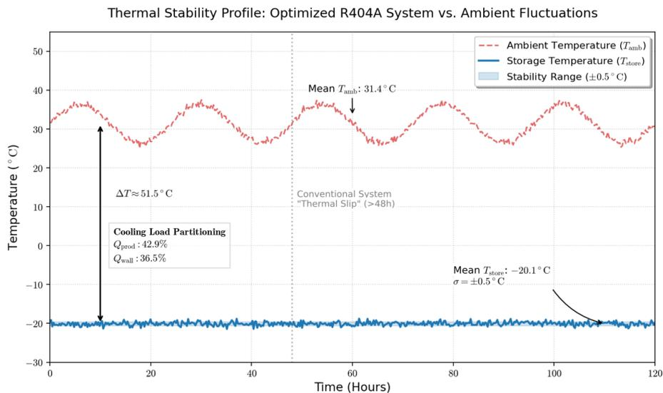
**Figure 2.** Thermal stability profile showing the correlation between ambient oscillations ( $T_{amb}$ ) and storage stability ( $T_{store}$ ) over the 120-hour voyage.
