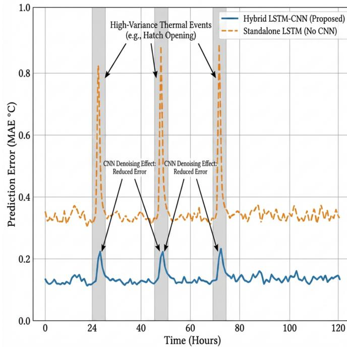
**Figure 6.** Impact of architectural ablation on predictive fidelity. The standalone LSTM (Orange, dashed) exhibits severe error spikes during high-variance events, whereas the proposed Hybrid LSTM-CNN (Blue, solid) effectively filters these transient noises through spatial convolution.
