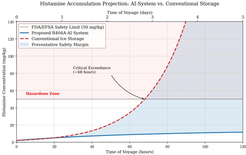
**Figure 5.** Histamine accumulation projection: Proposed R404A-AI System (Blue) vs. Conventional Ice Storage (Red dashed). The shaded area represents the preventative safety margin achieved by the AI framework.
